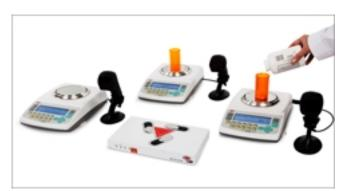
The server controls the DRX-500s pill counting stations and tracks all pill counting transactions as well as user activity. During each pill counting transaction the server sends the scale detailed information about the counted medication.
