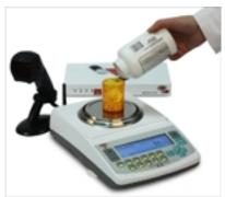
A typical pill counting transaction of 60 pills, performed on a DRX500 scale connected to the TORBAL server is made in three easy steps, and can be performed under 20 seconds. The steps are simple: tare the vial, scan the NDC located on the supply bottle, and fill the count. During each count the scale displays the name of the drug and other important drug information. Details of each transaction are logged by the server.
