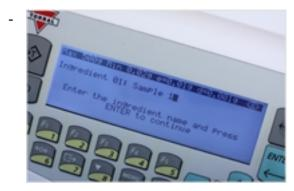
The large pixel type LCD display assists the user throughout the compounding function. Graphics and textual onscreen instruction guide the user through every step for greater ease and accuracy.
