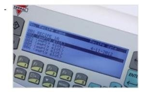
When compounding, the entire recipe can be stored in a library for later retrieval and viewing. The archived recipe includes date, time and the names and weights of each component ingredient.
