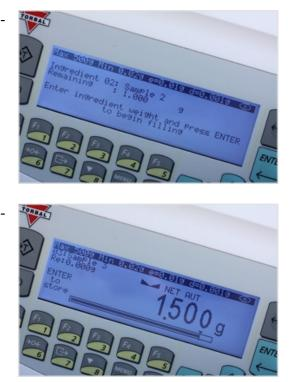
The Remaining To Fill display shows how much more weight is required to reach the desired weight. When this weight is keyed in, the scale tracks the filled weight and shows the remaining amount. If the user exceeds the desired weight, an excess indicator shows how much needs to be removed.
