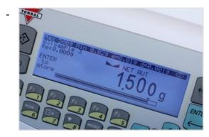
The Remaining To Fill display shows how much more weight is required to reach the desired weight. When this weight is keyed in, the scale tracks the filled weight and shows the remaining amount. If the user exceeds the desired weight, an excess indicator shows how much needs to be removed.
