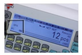
APA is an advanced pill counting algorithm that can adjust for production LOT pill weight variations and provide even greater accuracy when counting large quantities. The feature is very easy to use and requires little user interaction.
