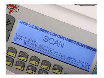
The large pixel type LCD display allows for graphics and full-text onscreen instruction to be displayed while counting pills. The pill counting function is designed as a short wizard that leads the user step-by-step through this simple operation. During the count the scale displays detailed drug information which is visibly organized on the scale's LCD.
