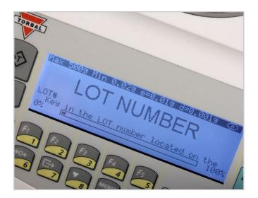
Labeling the drug with the actual name and LOT number is quickly and easily done via an external standard PC type keyboard connected to the scale's PS/2 port. The LOT number entry is particularly useful when maintaining drug's average piece weight. A small footprint PC type keyboard is offered as an accessory option.
