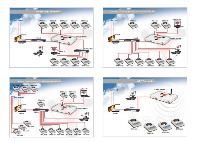
DRX-5 Workstations connect to the TORBAL Rx Server in four different ways. The Wi-Fi connection type offers a plug and play set up of the system. Wi-Fi scales are pre-configured to automatically connect with the TORBAL server wirelessly. This connection type is suitable in an environment where the scales are within 120' (32m) proximity of the TORBAL Rx Server and the wireless path is not obstructed by large or heavy structures.
