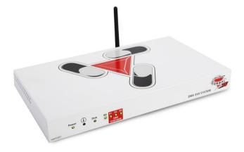
The WiFi configuration allows for a simple Plug-and-Play setup. The TORBAL server is designed to handle a network of up to 30 DRX500s pill counting scales. Scales can be connected directly to server, or through a hub or a switch of your existing local area network, as well as, a remotely over the internet.
