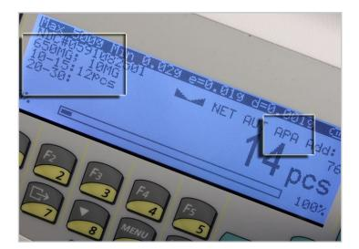
on the system server. This system not only improves counting accuracy, it also speeds up the process significantly and eliminates the need for the pharmacist to count pills manually when updating average piece weights.
