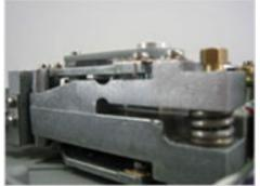
The heart of a quality is its load cell and suspension. The load cell should be of the electromagnetic force restoration type where the weight of the unknown is balanced out by the force generated by sending an electric current through a coil which is sitting in a high level magnetic field. The suspension should be of the Roberval type which compensates for end and side loads and allows the scale to be top loading.
