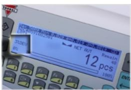
The Deviation Warning checks for discrepancies between a counted drug's average piece weight and its stored average piece weight and signals the user if a deviation above or below 2% is discovered.
